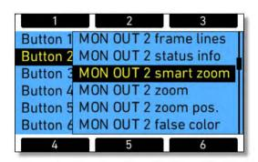
• An extra feature makes the ZOOM function on the EVF more convenient. When ZOOM is enabled on the EVF, rotating the EVF jog wheel steps through all zoom positions.
