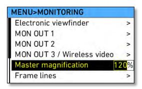
If less than the recorded area is shown on the EVF or on the MON OUT image, an orange border will be shown at the frame boundaries where the recorded image exceeds what is visible.
