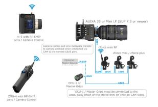
Connect the cforce mini RF to the camera via a CAM – LBUS cable and connect an OCU-1 or Master Grip to the motor LBUS daisy chain. Don't connect the LBUS side of the motor to the camera LBUS. Camera control and lens metadata are already transmitted via the CAM – LBUS connection.
