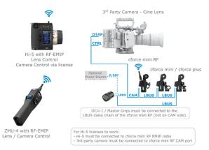
Connect the cforce mini RF to the camera via the according CAM cable and connect an OCU-1 or Master Grip to the motor LBUS daisy chain.
