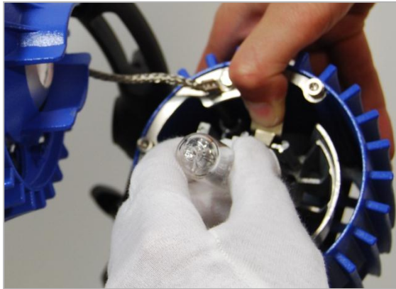
7 Pull the lamp retainer aside again and insert the new lamp carefully into the lamp holder holding the lamp at its socket.
