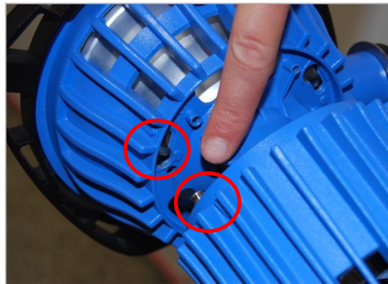
11 Make sure that the guide pins of the lamphousing (3 in total) slip into the holes of the reflector housing (3 in total). Be careful that the grounding strap is not squeezed.
