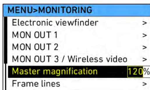
If less than the recorded area is shown on the EVF or on the MON OUT image, an orange border will be shown at the frame boundaries where the recorded image exceeds what is visible.
