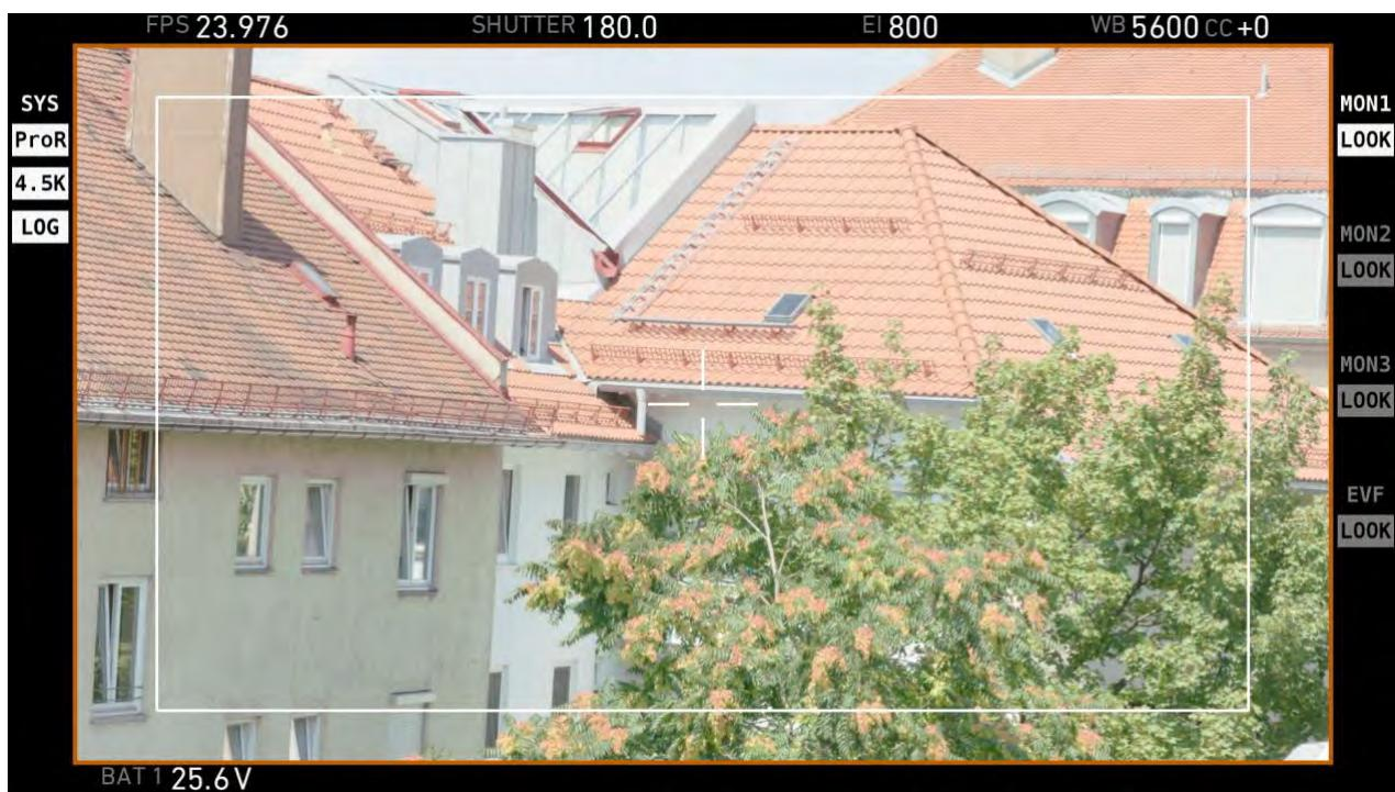
A screenshot from an ALEXA LF in LF Open Gate Mode with a 16:9 frameline (white rectangle). To enlarge the image on the monitor, the MAGNIFICATION feature has been used. The orange borders indicate that more image is being recorded than is visible.
