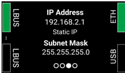
7 Configure the NIA-1 from DHCP mode to a static IP address within the same subnet (e.g. 192.168.2.1). The first three digits of the NIA-1 IP address (network address) shall be identical with the camera IP address.
