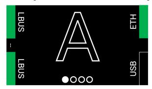
The outlined Network Channel symbol indicates that the channel is set, but no connection is established over the Ethernet port to at least one NIA-1 with an identical Network Channel.
