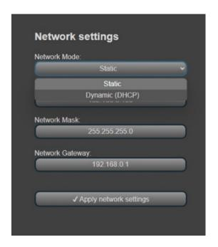
Now, both CSS IP-Boxes can be connected to a local network and they will connect automatically. The assigned IP address is now visible on the display of the CSS IP-Box, as shown and can be entered again in a web browser to configure the CSS IP-Box.
