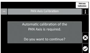
As soon as the Pan Axis module is connected to the TRINITY Head, supplied with suitable power and the TRINITY Head is switched on, the autocalibration of the system starts automatically.
