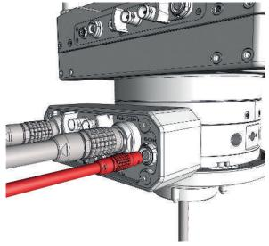
Finally, connect the FS CAN cable to the Junction Box and the RCP-3 with the FS CAN cable.
