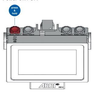
To turn the RCP-3 on and off, press and hold down the jog-wheel until the ARRI logo appears or disappears on the display.
