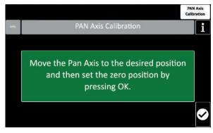
After completing the calibration, the Pan Axis needs to be set to the desired zero point / home position. To achieve this, simply turn the TRINITY remote head to the desired position and touch OK. As a guide, we recommend positioning the TRINITY Remote Head 90 degrees to the junction box.
