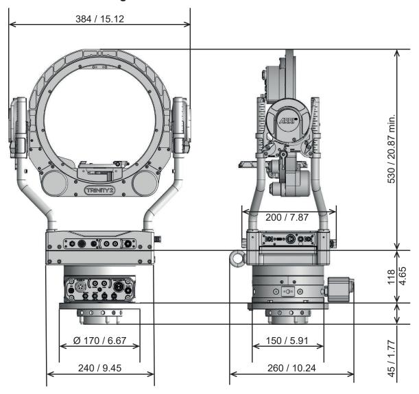
All dimensions given in millimeter / inch. Drawing not to scale.
