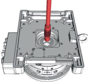
Guide the main cable from the top through the Pan Axis Module.
