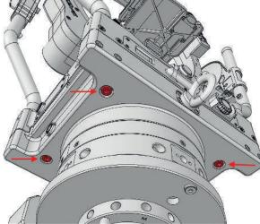
• Use a 5 mm Hex key to tighten the four screws.
