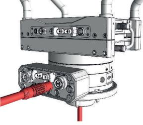
Plug the Main Cable into the Junction Box after the Mitchell Mount has been mounted on a crane or dolly.
