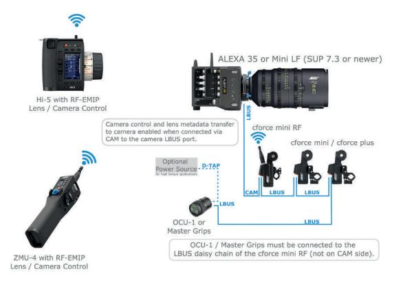
2) OCU-1 with a cforce mini RF as a radio host on an ALEXA 35 or ALEXA Mini LF (SUP 7.3 or newer)
