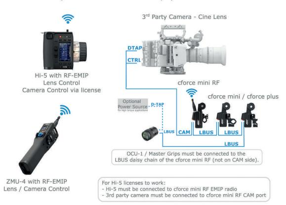
8) OCU-1 with a cforce mini RF as a radio host on a 3rd party camera with cine lens
