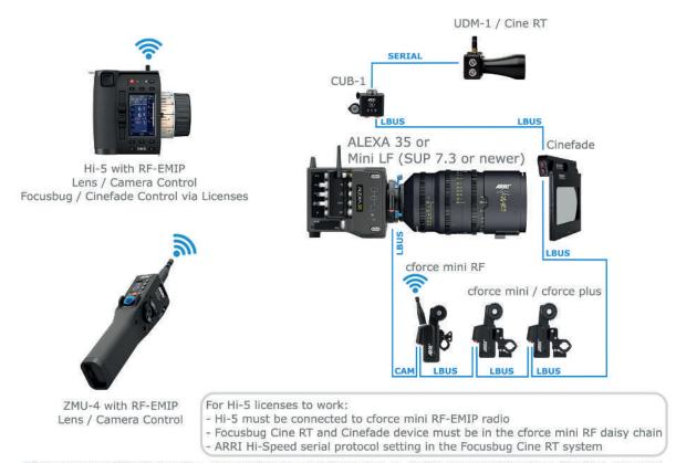
3) Focusbug and Cinefade with a cforce mini RF as a radio host on an ALEXA 35 or ALEXA Mini LF (SUP 7.3 or newer)
