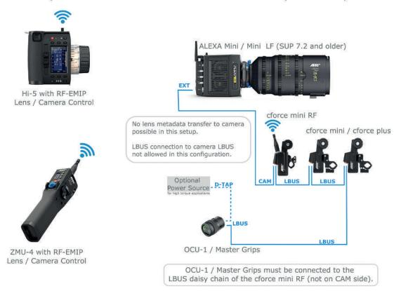
5) OCU-1 with a cforce mini RF as a radio host on an ALEXA Mini or ALEXA Mini LF (SUP 7.2 or older)
