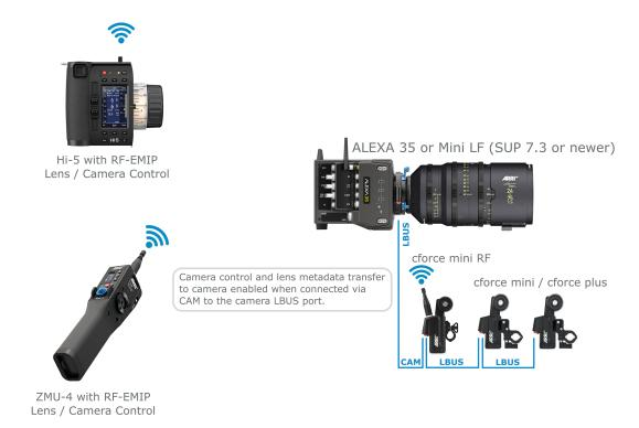
1) cforce mini RF as a radio host on an ALEXA 35 or ALEXA Mini LF (SUP 7.3 or newer)
