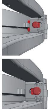
TILT Lock OUT Before switching ON the remote head, the TILT lock must be deactivated!
