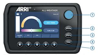
Illustration 4: Control elements of the control panel
