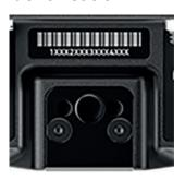
The CCM-1 serial number is located on the product label in the lower center of the CCM-1.
