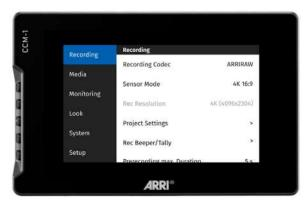
The CCM-1 offers access to the complete camera menu for access to all camera settings.
