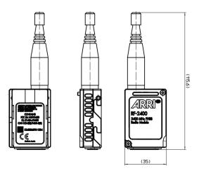
Weight of the RF-2400 Radio Module: 52g/1,83oz (including antenna)
