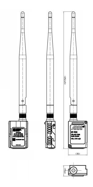
Weight of the RF-900 Radio Module: 55g/1,94oz (including antenna)
