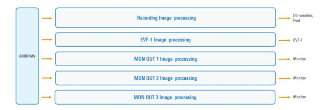
To maintain the highest overall image quality, all ALEXA in-camera image processing starts out with the uncompressed and unencrypted ARRIRAW data. This data goes through a recording image processing path and gets recorded, either as ARRIRAW or as ProRes. It is then used for creating offline deliverables like dailies and editing proxies and for further online postproduction like VFX and final grading.
