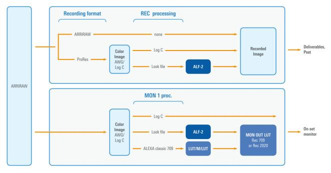
To gain a better understanding of the monitoring image path, we take a look at MON OUT 1, one of the four monitoring image paths. MON OUT 2 and MON OUT 3 function exactly the same. First, the ARRIRAW data goes through a debayering step and an AWG/Log C color image is created. What happens next depends on the choice made in the "MON 1 proc." menu of the "COLOR > EVF/MON PROCESSING" screen.
