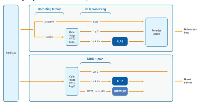
If you choose Log C in "MON 1 proc.", the Log C image is not processed any further, and is fed directly to the MON OUT 1 output. Since AWG/Log C is a virtual color space, there is no meaningful definition for how it should be displayed, and therefore we do not offer the option of transforming the image for Rec 709 or Rec 2020. AWG/Log C images will look more saturated on a Rec 2020 monitor than on a Rec 709 monitor.
