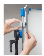
With the pole holes pointed outward from the fixture slide the metal bracket over the front of extrusion on the SkyPanel. This should hook in between the front of the fixture, and the metal extrusion. The metal blocks will then hook around the rear of the extrusion. Tighten the thumbscrews, ensuring the bracket is secure.
