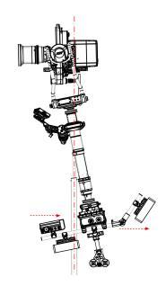
Open the 19mm rod clamp at the battery hanger and move the entire assemble (rods, batteries and the RCP-3) fore or aft till the entire rig reaches a
