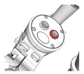
► Connect the 12G HD SDI BNC Cable, 0,63m/25in (K2.0041984) with the Monitor Out at the TRINITY 2 head and the Video In of the monitor.
