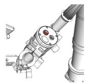
Connect the TRINITY 2 Joystick Cable 75cm/29.5in (K2.0043861) with the lower LBUS Socket at the Master Grip TRINITY and with the LBUS Socket at the TRINITY 2 head.
