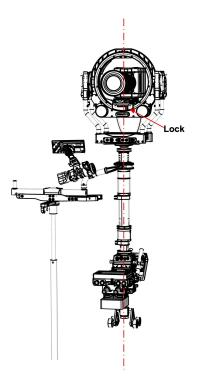
► To verify that the entire system is **neutral** in the **vertical axis**, check the bubble at the top stage.
