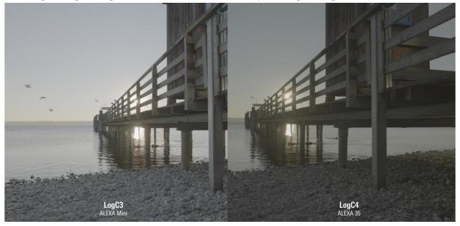
LogC4 is very different from LogC3 (the Log C you are used to)! This calls for adaption when exposing the sensor as a single operator as well as for DITs who monitor exposure or do live grading. LogC3 3D LUTs do NOT work with LogC4 and may lead to unwanted results!
