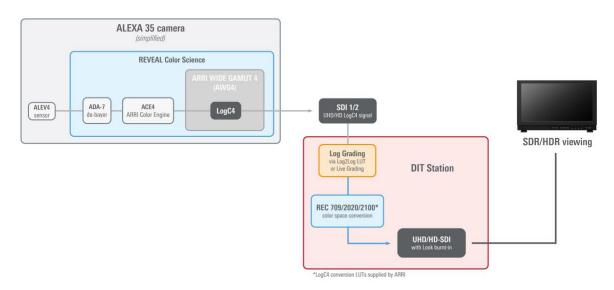
ALEXA 35 Look/LUT Workflow on-set with external LUT box/grading - not using ALF4
