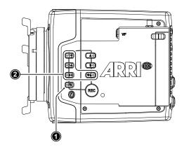
The camera's left side is equipped with the function button FN (1) and six camera buttons of which four are labelled with additional icons (2). These four buttons can act as regular user buttons or in combination with the FN button access common camera functions.
