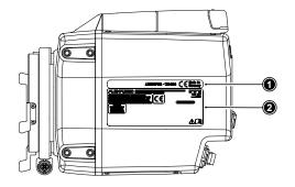
The camera serial number (1) and the FCC/CE conformity label (2) are located on the bottom of the camera. The serial number consists of the last 5 digits of the product number K1.0024074-XXXXX.
