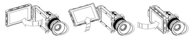
Fold out, swivel and fold in the monitor to put the display visible in the folded-in position. The image on the monitor automatically adjusts its orientation, or can be set to the desired orientation in the camera menu).
