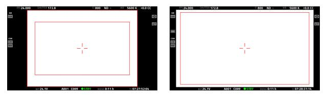
Two screen shots from an ALEXA Mini LF in recording resolution *LF Open Gate 4.5K* with a 1.78 UHD frame line (red rectangle) applied. The left screen shot shows the SDI output without magnification applied. The right screen shot shows the SDI output with magnification applied to enlarge the image (in this example set to 135%).
