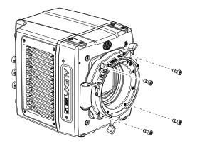
3. Crosswise, hand-tighten all four lens mount screws with a 3.0 mm Allen key.
