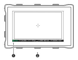
Use the lower screen buttons (2) to change the status bar (1) content. The lower center screen button returns to display the main camera parameters.
