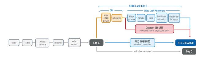
A look file can be created in the <u>ARRI Color Tool</u> as a completely new look, using a 3D LUT created in a grading session or you can edit the look live on set using a live-grading application like Filmlight Prelight or Pomfort Livegrade. For a more detailed look at a specific live-grade workflow, please visit the manufacturer website.
