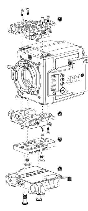
Using a 3.0 mm Allen key, fasten the Mini Adapter Plate MAP-2 or MAP-2A (1) to the camera top attachment points with the four 3.0 mm hex screws. Tighten them crosswise.
