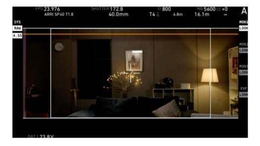
From ALEXA LF SUP 4.3 on, if less than the recorded area is shown on the EVF or on the MON OUT image, the orange line will not be shown any longer. Instead, new warning icons will be shown in the status area to the right of the image. See the table and image below for details.
