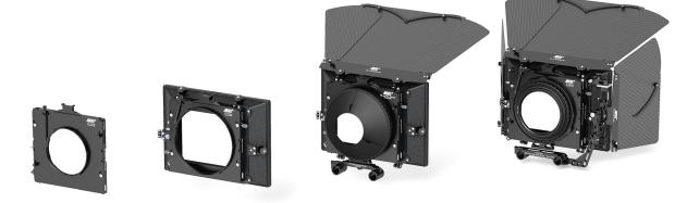
The LMB 6x6 is designed for maximum modularity at a minimum weight, and can be fitted without the use of tools. Optimized for up to three 6.6 x 6.6 inch filters, the LMB 6x6 can be used with 15 mm and 19 mm studio rod support.
