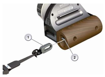
1. Insert the shoulder strap's snap hook (1) into bottom eyelet (2).
