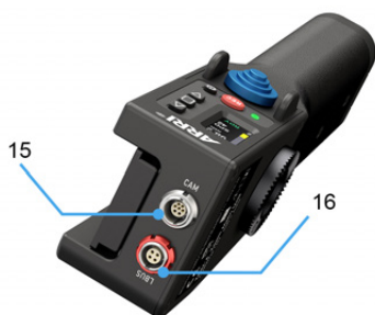
15 CAM interface 16 LBUS interface
