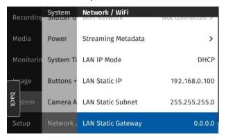
In certain setups, especially for virtual productions, there is a need to define a network static gateway. The default static gateway is a router that forwards network packets when no other route matches the destination of a packet. In a local network, the default gateway is typically the host that is one hop closer to the internet. The IPv4 address of the gateway typically is the first address in a subnet, e.g. 192.168.0.1. As a factory default the gateway is set to 0.0.0.0.
