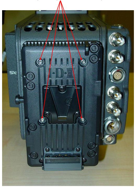
This completes the installation of the V-Mount Adapter Back To perform a functional Test, see Chapter 13.
