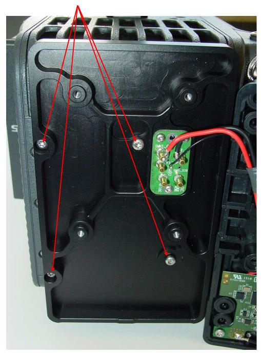
Make sure that the mounting frame for the V-Mount Adapter is firmly attached to the camera.
