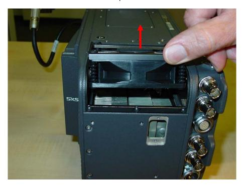
Carefully disconnect fan cable using tweezers and then remove the fan completely.
