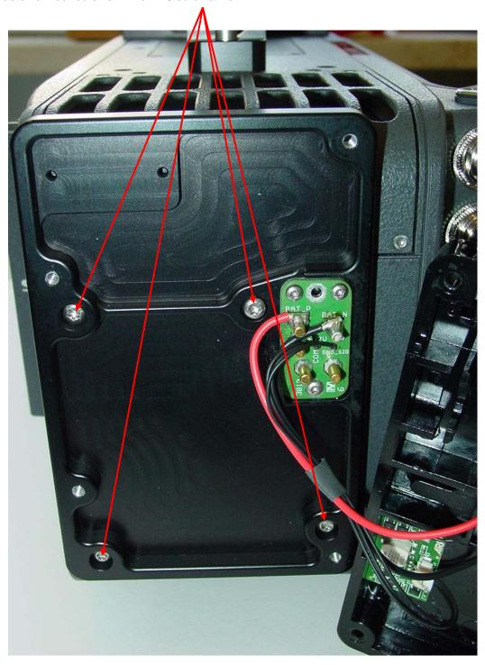
Make sure that the mounting frame for the Gold-Mount Adapter is firmly attached to the camera.
