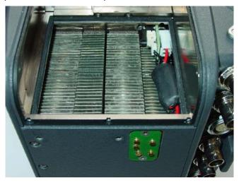
Fix plastic cover on the connector PCB with the two M2x5 screws, using a TX6 screwdriver.
