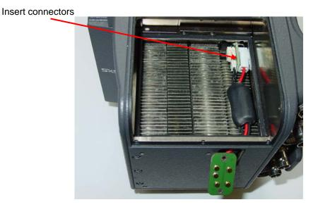
Align cables and push connector PCB in place.
