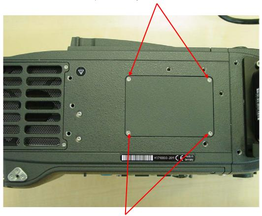
Remove all four screws completely.
