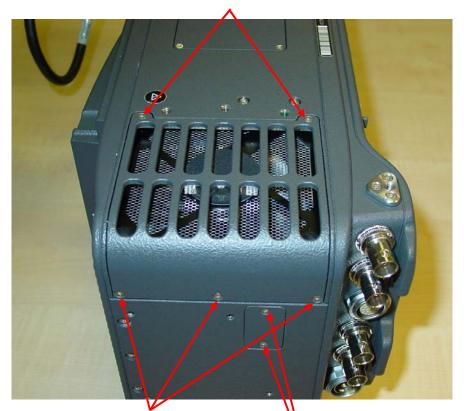
Do not remove the screws completely. Then take fan cover away.
