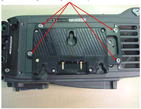
This completes the installation of the Gold-Mount Adapter Top. To perform a functional Test, see Chapter 13.
