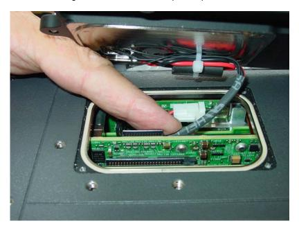
Then tighten the 4 mounting screws using 3mm Allen key.
