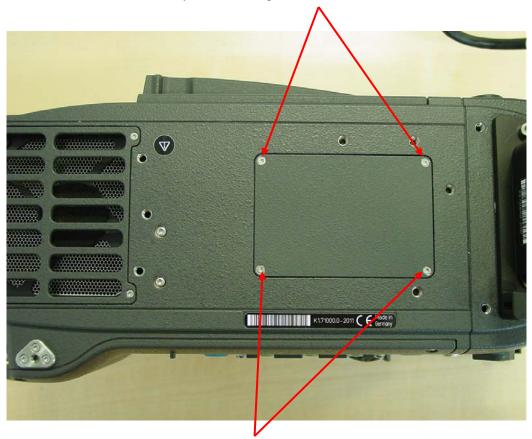
Remove all four screws completely.
