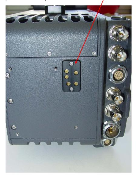
This greatly simplifies the changing of back mount battery adapters in the field. All back mount battery adapters ordered separately, will be supplied with the required new connector for retrofitting existing cameras.
