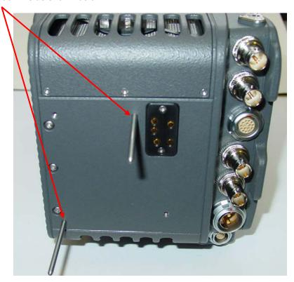
Push the mounting frame over the Guide Pins to its correct position and then secure it by using two of the four screws M3x8, as shown.
