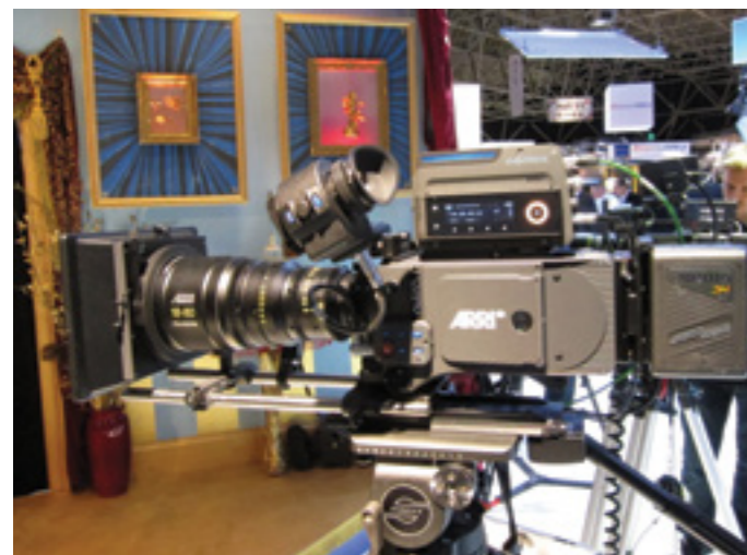
ALEXA Plus with Codex Onboard Digital Recorder, ARRI/Fujinon Alura 18-80 mm zoom, Anton/Bauer onboard battery.
