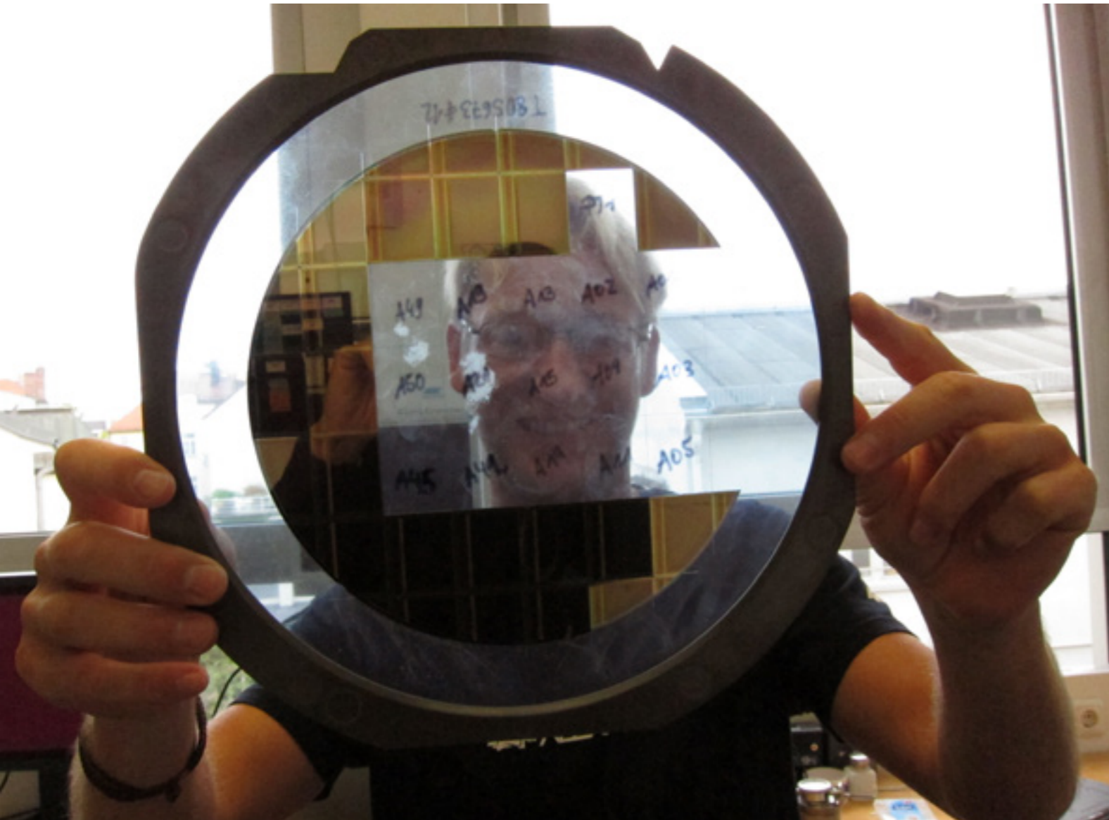
Above: sensors arrive from the foundry on a flexible carrier, arranged like a circular tray of ice cubes. They must be cut apart, mounted, connected and protected by a low pass filter pack, below.
