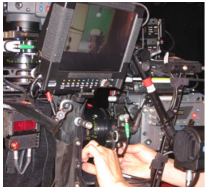
Chosen for "Hugo Cabret" because of high sensitivity (800 EI) and dynamic range
