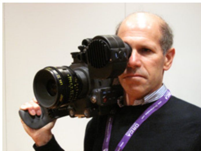
Cooling. That was an interesting subject. The internal electronics are totally sealed against dust, salt, spray and dirt. Heat is blown away from the sealed capsule with a quiet, replaceable 20 db fan. Since the bearings of a fan motor are usually the first thing to go, you can pull out the entire fan and replace it with a new one. Because the electronic compartment is sealed, the fan is only blowing against a "radiator" that collects the heat from inside the electronic's compartment, and not blowing salt water, sand or dust onto sensitive components.
