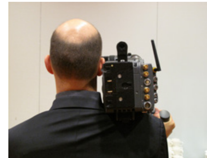
Smaller and lighter than an ARRICAM Lite. Anton/Bauer and IDX style 14 volt on board batteries can be used. The camera will automatically switch between the 24V and the 12V power inputs. We noticed 12 volt and 24 volt accessory receptacles. Monitoring will be flicker-free, courtesy of image frame-store technology.
