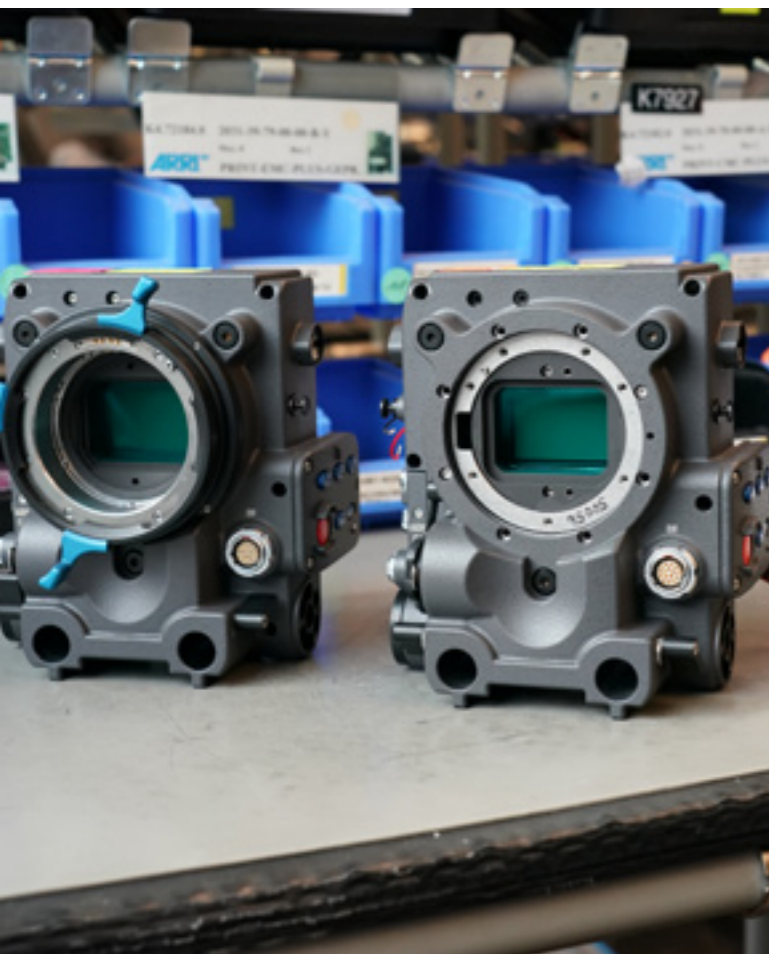
Sensor assemblies installed. Attach LPL mount to camera body on left.
