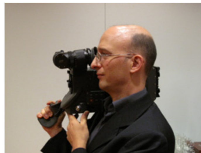
Smaller and lighter than an ARRICAM Lite. Anton/Bauer and IDX style 14 volt on board batteries can be used. The camera will automatically switch between the 24V and the 12V power inputs. We noticed 12 volt and 24 volt accessory receptacles. Monitoring will be flicker-free, courtesy of image frame-store technology.
