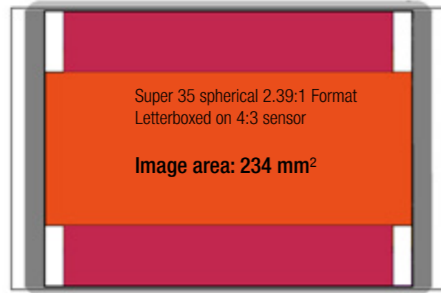
Fig 1. Spherical 2.39:1 on 4:3 ALEXA Sensor
