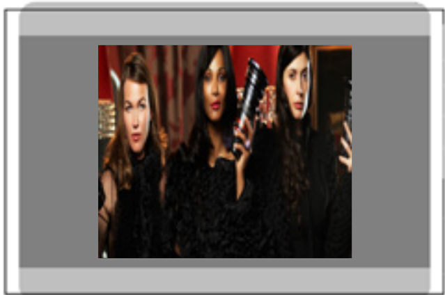
16:9 Sensor with same lens and same 2x squeezed image: the smaller sensor size crops image by a factor of 1.8x and Linda gets a haircut
