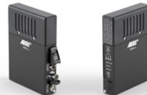
ARRI WVR-1s Connectors: Power IN (10.5-34 V DC) 2-pin Lemo Power OUT (12 V DC, max 2.0A) 2-pin Lemo 3G-SDI OUT BNC
