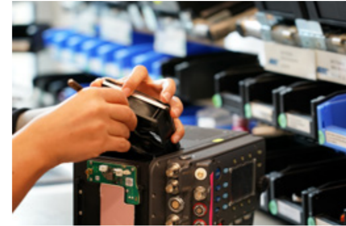
The cooling fan goes in.
