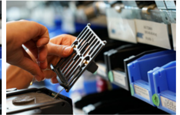
Fan cover is attached.
