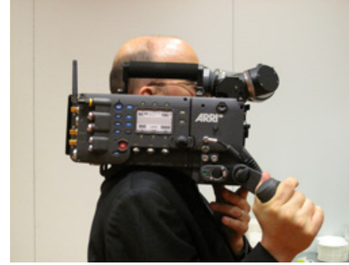
The optical modules of the Alexa OV-Plus add a few inches to the front of the camera. Notice the extra area around the ARRI logo and the familiar bulge of the mirror shutter. There's no room for molded 15mm lightweight support holes. Also, notice that the OV camera includes the "Plus" features of wireless remote camera and lens control—identified by the rear antenna and the lens motor receptacles.
