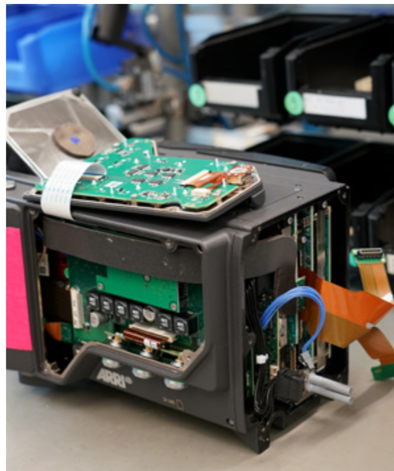
Printed Circuit Boards and fan go inside the rear camera body housing.
