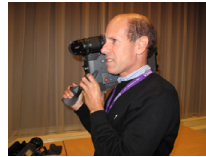
There's a convenient handgrip rosette on the camera right side. I hope there will be a handgrip rosette on the left side as well—as it is on the Arriflex 16SR. The optical finder will swing over to either side of the camera body, and extends in and out like an Arriflex 435.
