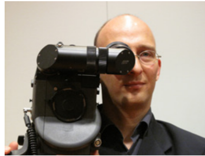
The optical modules of the Alexa OV-Plus add a few inches to the front of the camera. Notice the extra area around the ARRI logo and the familiar bulge of the mirror shutter. There's no room for molded 15mm lightweight support holes. Also, notice that the OV camera includes the "Plus" features of wireless remote camera and lens control—identified by the rear antenna and the lens motor receptacles.
