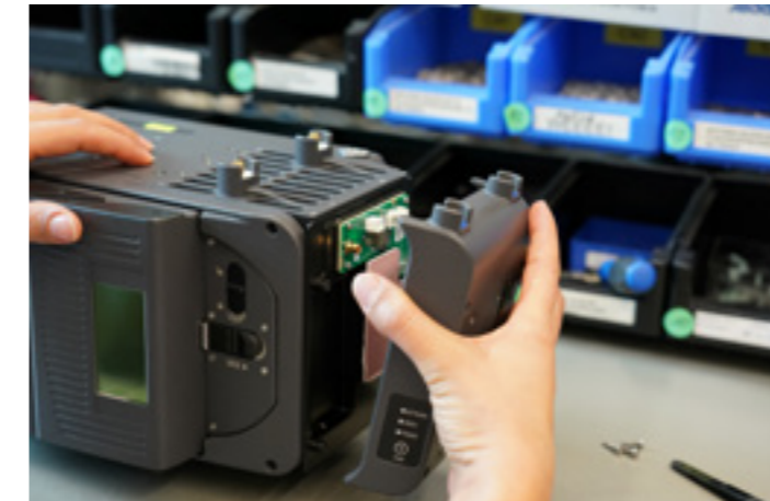
Wireless video module goes on the back.
