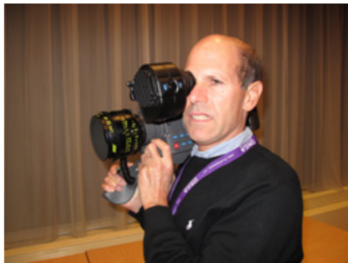
The electronic viewfinder model shown here (EV) is lighter and smaller than the optical viewfinder (OV) model on the opposite page. Essentially, the basic cameras are similar, but the OV version adds a spinning mirror and optical finder assembly in front. The electronic finder attaches to many places around the camera, depending on your operating needs: front, rear, right side, and so on.
