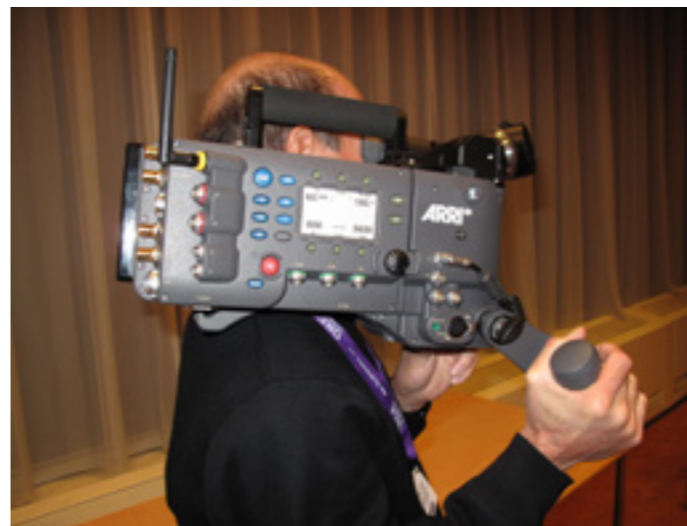
There's a convenient handgrip rosette on the camera right side. I hope there will be a handgrip rosette on the left side as well—as it is on the Arriflex 16SR. The optical finder will swing over to either side of the camera body, and extends in and out like an Arriflex 435.
