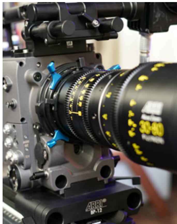
PL-to-LPL adapter accepts any PL mount lens on ALEXA LF. The PL mount has 2 traditional black ears. The LPL mount has 3 blue ears.
