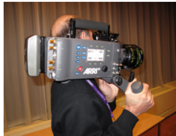
The electronic viewfinder model shown here (EV) is lighter and smaller than the optical viewfinder (OV) model on the opposite page. Essentially, the basic cameras are similar, but the OV version adds a spinning mirror and optical finder assembly in front. The electronic finder attaches to many places around the camera, depending on your operating needs: front, rear, right side, and so on.
