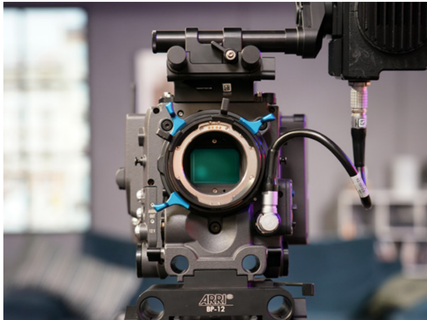
PL-to-LPL adapter accepts any PL mount lens on ALEXA LF. The PL mount has 2 traditional black ears. The LPL mount has 3 blue ears.
