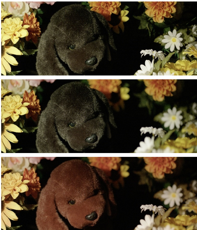
Figure 1. Upper image: No filter. Middle image: ARRI FSND 1.2 filter. Lower image: Typical classic dye based ND 1.2 filter (not IRND). A neutral density filter enables smaller T-stop settings while keeping exposure constant, to blur the fore- and background due to a decreased depth of field. For example, a scene that is exposed with a T-stop of 5.6 (upper image) can be exposed at 1.4 (+4 stops); when a ND 1.2 filter (-4 stops) is implemented (middle and lower images); when using digital cameras, attenuation of near-infrared light becomes essential to avoid false color issues (bottom image).
