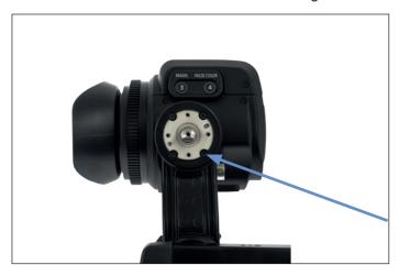
5. Unscrew the 4 screws and remove the clamp hinge and the clamp hinge base
