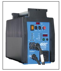
For high-speed operation three different modes are available: AutoScan (fully automatic), Man (manual frequency control) or AutoMan (combining manual frequency setting with automatic frequency control). Using the AutoScan mode requires no further interaction by an operator. After a two-stage scan the lamp frequency is selected and set by the ballast; all parameters are continuously monitored and adjusted automatically if required.
